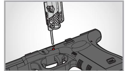
Easily remove all pins to disassemble your Glock to clean, modify or maintain
