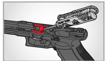
Remove & install internal components like the slide lock spring & locking block with small flathead driver
